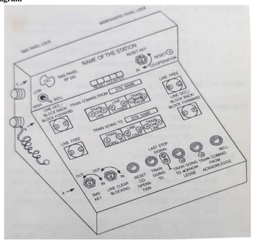
The running of every train shall in its direction from one block station to another on double line be regulated by means of a block panel with associated axle counter and other equipments.
