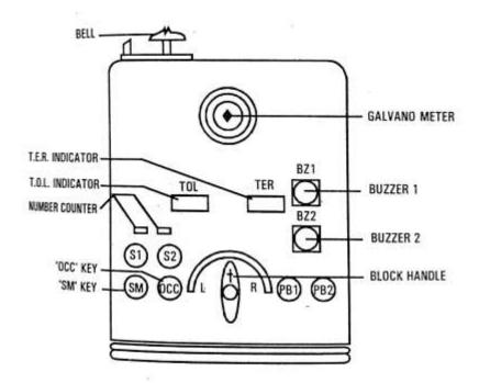
The Block Instrument has the following controls and indications as shown in the sketch:
